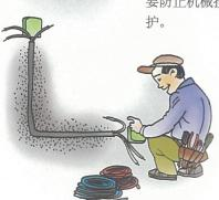
Avoid the wires touching or approaching the combustible materials when electrical wiring. Avoid the wires being exposed to sunshine or rain to wear. Electrical wires should be protected by casing pipe. When surface wiring, avoid the mechanical damage. When passing through floors or walls, electrical wires should be protected by porcelain pipes or steel pipes.
